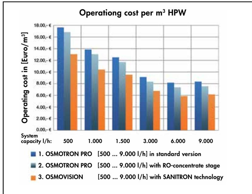
Fig. 7: Comparison of specific operating cost per m³ Highly Purified Water.
