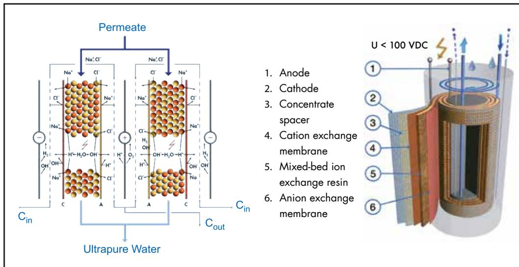
Fig. 1: Elementary diagram and structure of electro-deionization for a helical winding module (SEPTRON®-Module); Source: All illustrations BWT Pharma & Biotech GmbH, if not specified otherwise.
