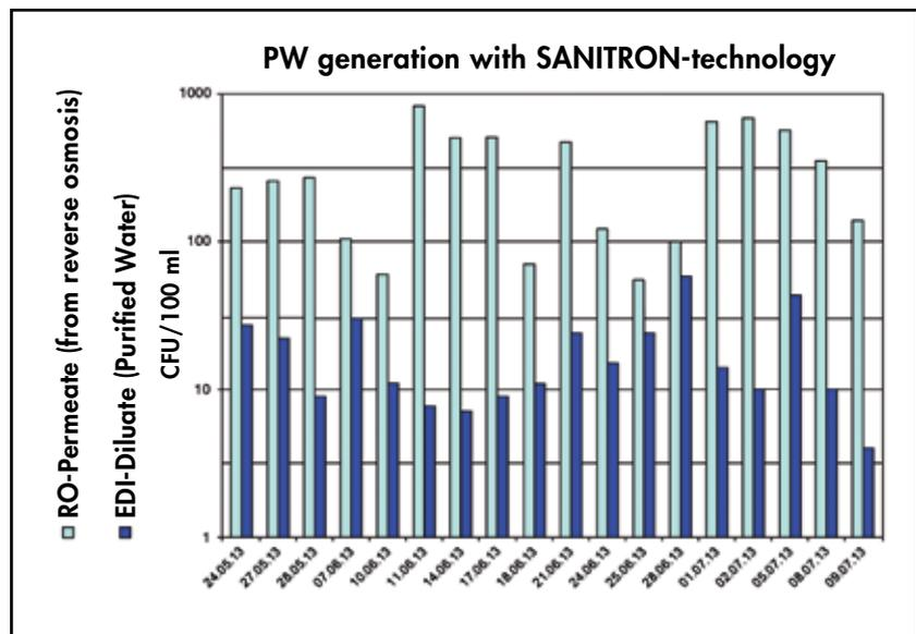
Fig. 5: Cfu values in RO-Permeate and EDI-Diluate (Purified Water) of a PW production plant equipped with SANITRON-Technology (with SEPTRON®-EDI-Module, without BioSafe-Ultrafiltration-Membrane Unit).
