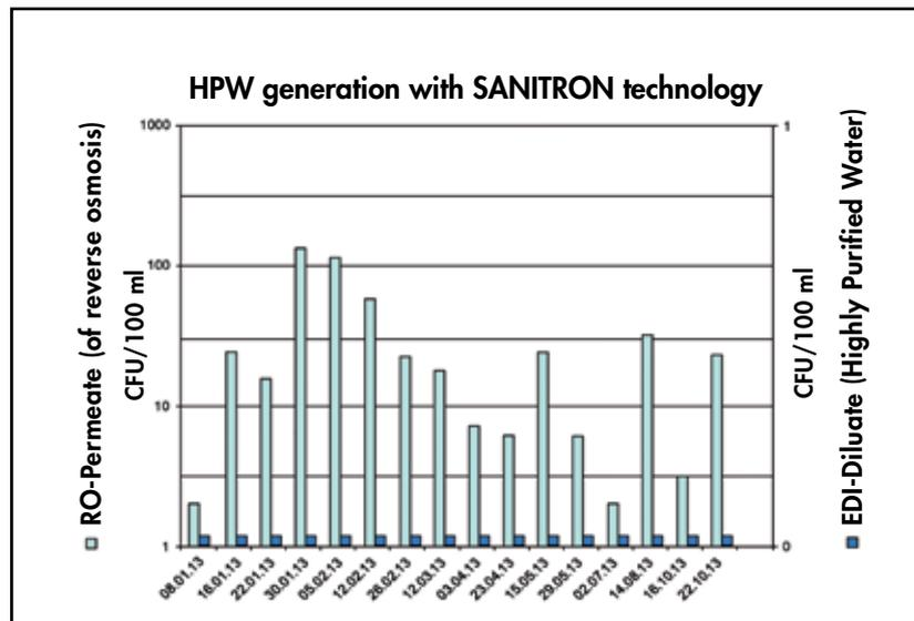
Fig. 6: CFU values in RO-Permeate and EDI-Diluate (Highly Purified Water) of a HPW production plant equipped with SANITRON-Technology (featuring SEPTRON®-BioSafe EDI-Module).
