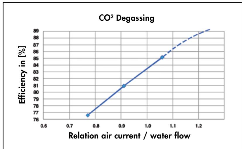
Fig. 3: Efficiency of CO<sub>2</sub> degassing depending on the relation air current / water flow for a CO<sub>2</sub> concentration of 50 ppm in water.
