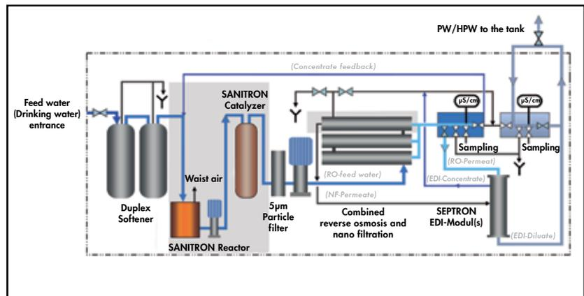
Fig. 4: Elementary diagram of the SANITRON-Technology.
